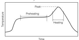
For soldering (Example: Sn/Pb)
